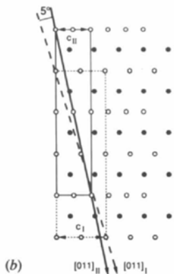
Fig. 9. (a) Reciprocal lattice sections I and II of the compound (\text{CaSr})_{14}\text{Cu}_{24}\text{O}_{41} ; (b) corresponding direct lattice directions.
